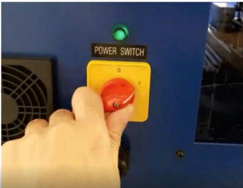
1. Turn on the power switch on the control panel. The power switch will light up when on.
