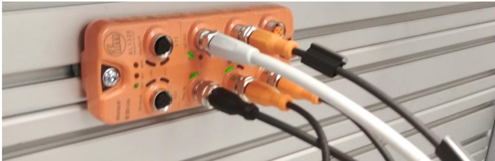
An IO-Link master device mounted onto the JMETS
