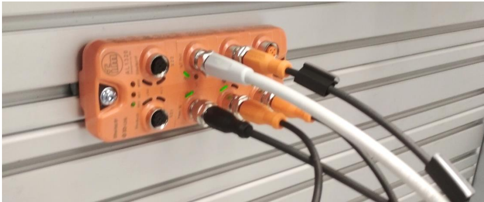
An IO-Link master device mounted onto the JMETS.
