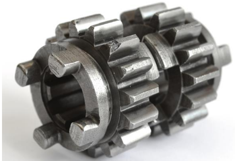
A damaged gear tooth
