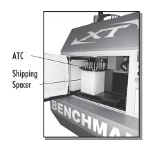
From inside the XT: Ease the ATC down onto the styrofoam spacer, and check to make sure it is centered firmly on the spacer.
