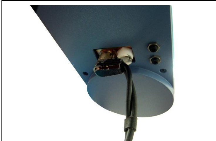
Figure 4: Connecting Gripper Cable to SCORBOT-ER 14 Pro
