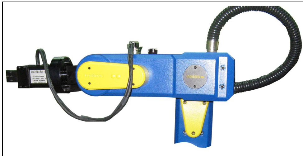
Figure 2: Connecting Gripper Cable to SCORBOT-ER 9Pro
