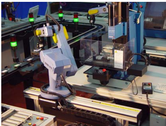
Figure 17: FMS with Prolight 1000, LSB 1.8 and ER-IX
